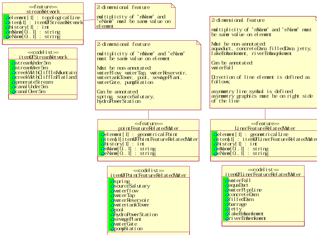
Figure 3: UML diagram of the “hydrography” package
