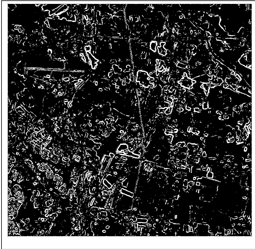
Figure 5. Fragment of image boundaries by Hueckel operator with window 5x5, conf=0.8 and diff=0.4.
