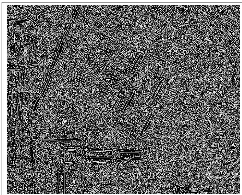
Figure 12. Object boundaries obtained by Canny detector with \sigma=0.9 , t_{high}=0.9 and t_{low}=0.3 .
