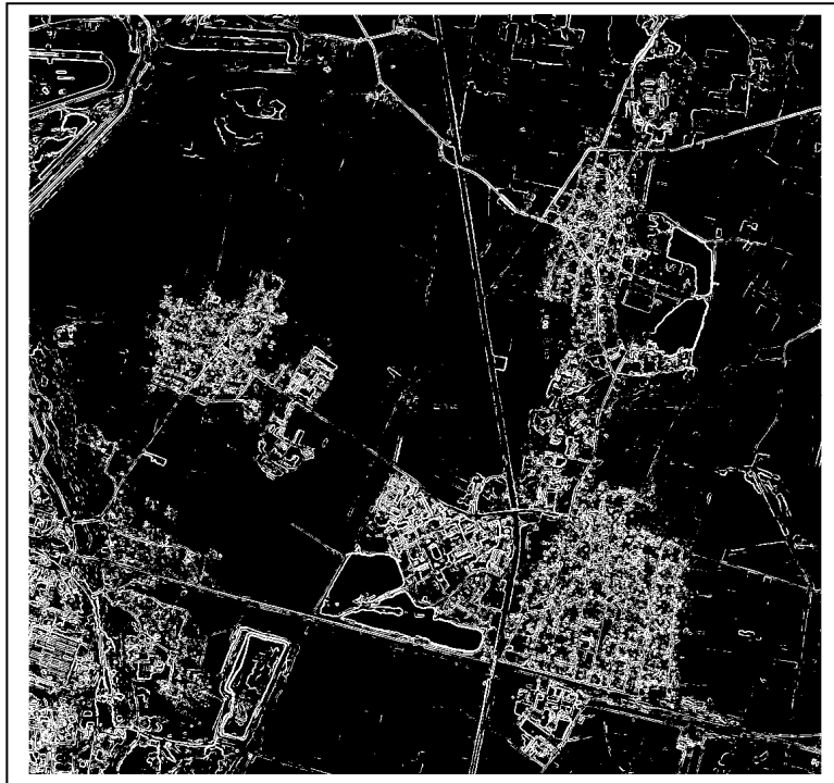
Figure 7. Fragment of boundary map after applying the Sobel operator with threshold level t=42 .
