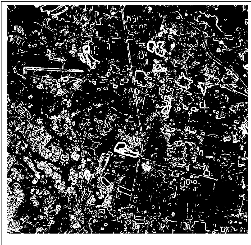
Figure 4. Contour elements after Sobel with window size 3x3 and threshold 9.
