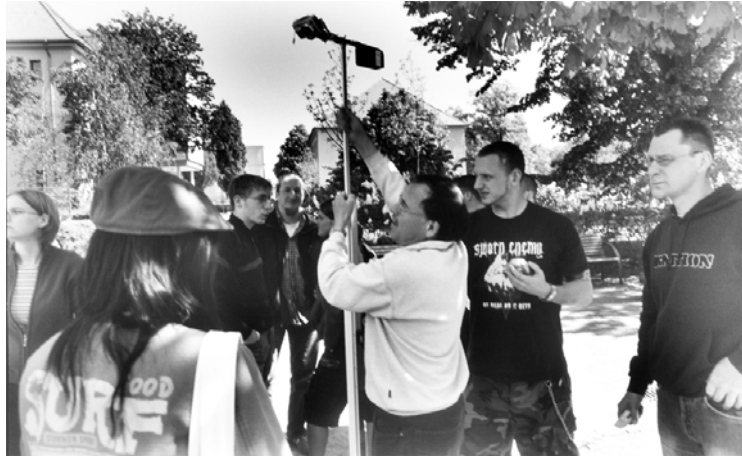
Figure 9. Dipl.-Eng. St. Kiel of the University of Applied Sciences Magdeburg - Faculty of Civil Engineering- demonstrating a single lenses version of his digital 3D staff camera with remote control.
