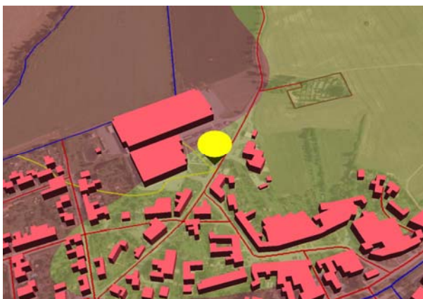
Fig. 8: More realistic 3D area model presenting simulated accident site location (yellow cone), estimated liquid pollutant runoff routes (yellow lines), closest water objects (blue lines), differentiated pollutant infiltration risk areas (lower risk – green, higher risk – purple), land use structure (orthophoto) and buildings – information given is applicable especially for DM staff
