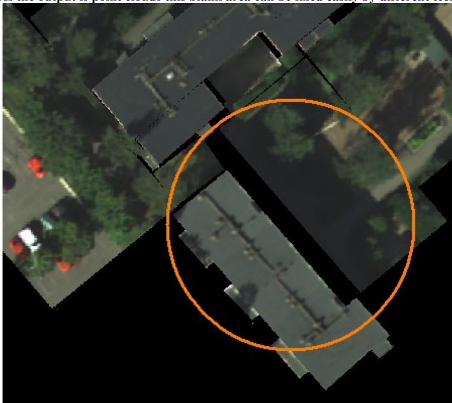
Figure 6: The output of registration of the colour image on the Optech laser scanner data. Same Figure 5 the effect of relief displacement has been omitted in this output.
