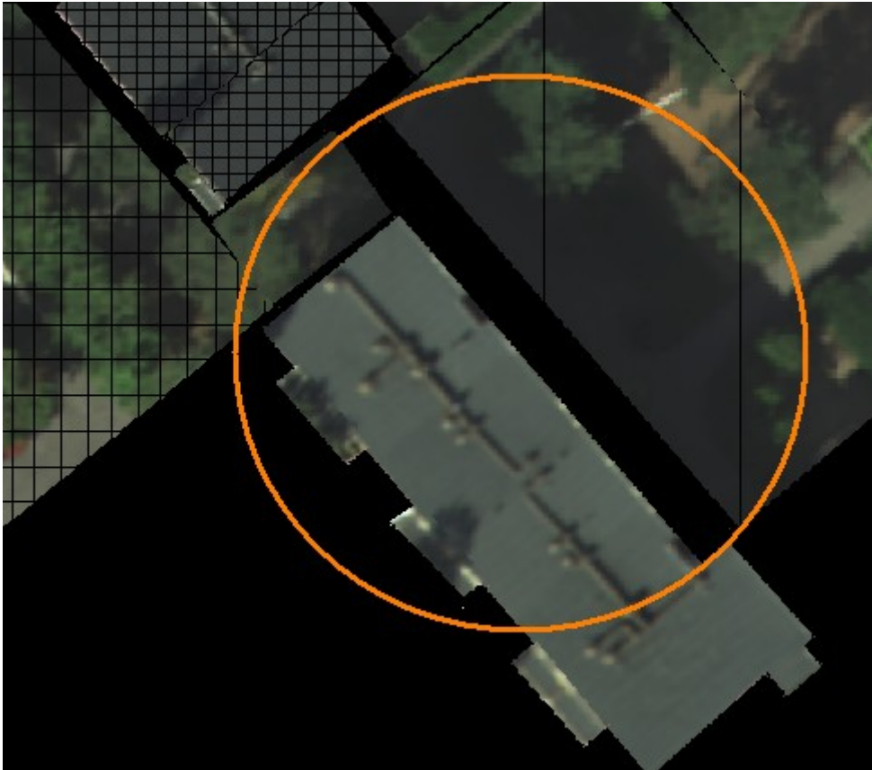
Figure 7: The output of registration of the colour image on the combined laser scanner data. It can be seen that the effect of relief displacement has been omitted.
