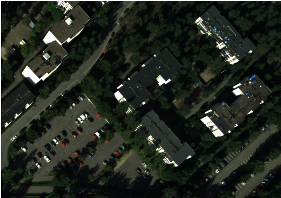
Figure 4: Original image from one of areas which have been chosen for image registration. The relief displacement's effect on the image can be easily recognised. The facial of buildings can be seen.
