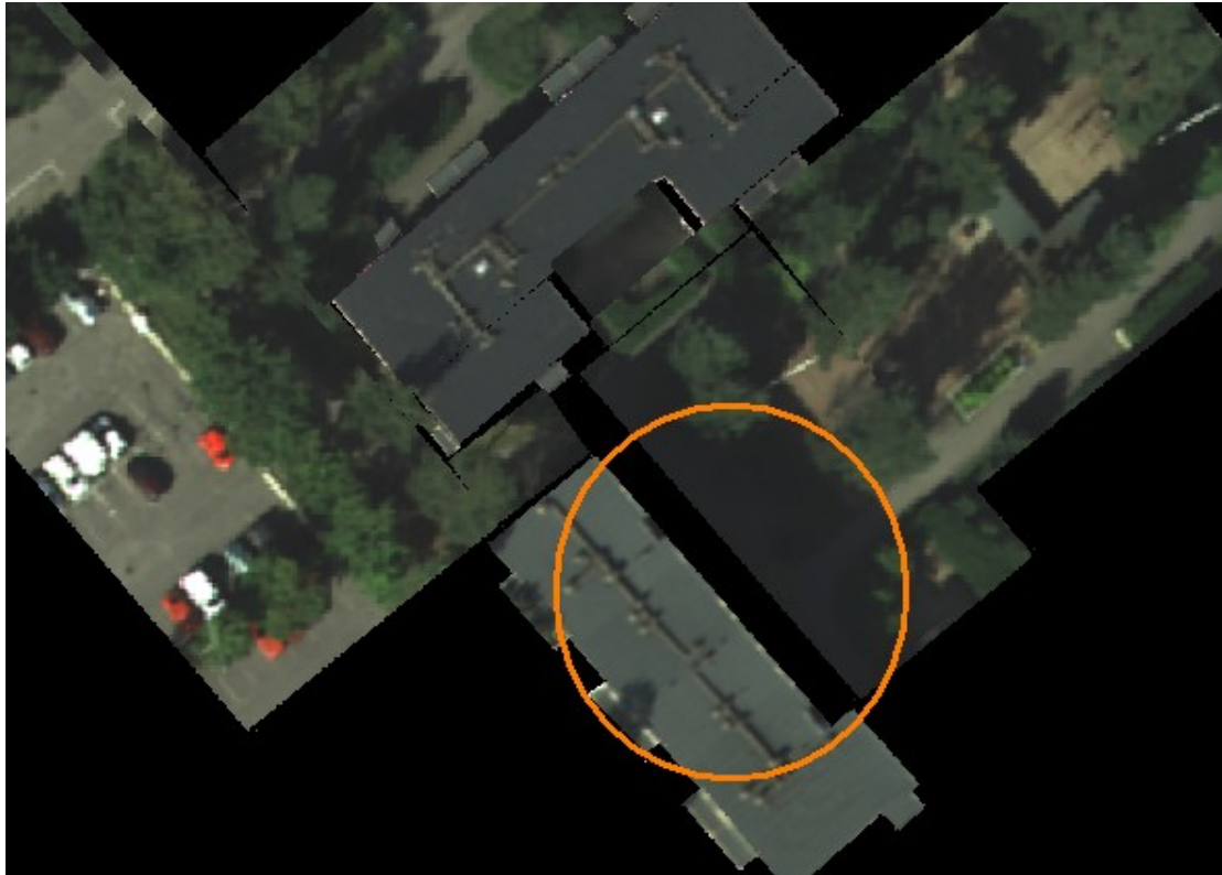
Figure 5: The output of registration of the colour image on the Leica laser scanner data. The blank area in the red circle indicates that the relief displacement has been omitted because image of building was pulled back and rectified consequently a blank area appears in the output in the place. As the output is point clouds this blank area can be fixed easily by different techniques.
