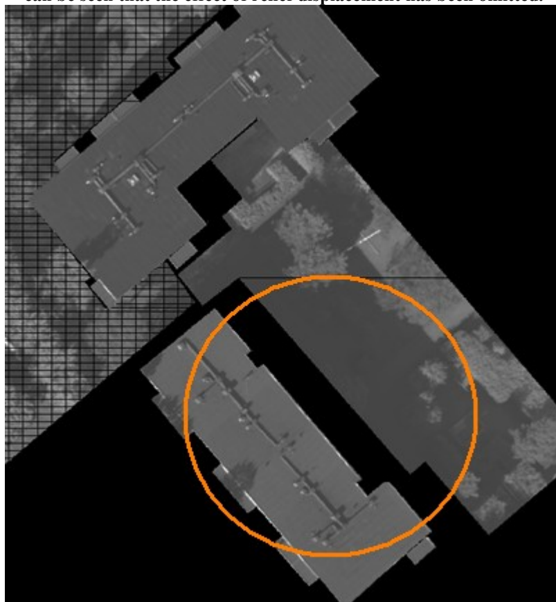
Figure 8: The output from registration of the panchromatic image on combined laser scanner data. It can be recognised that relief displacement has been fixed.
