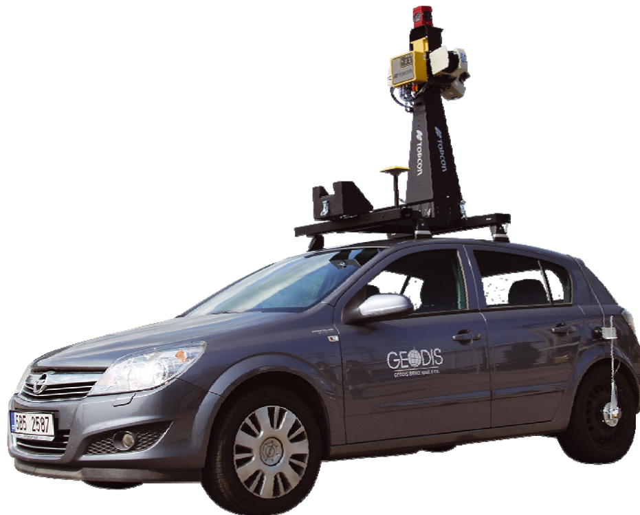
Fig. 1 Basic IP-S2 mobile mapping system configuration
