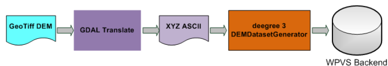
Fig. 8: DEM to deegree3 data conversion toolchain.
