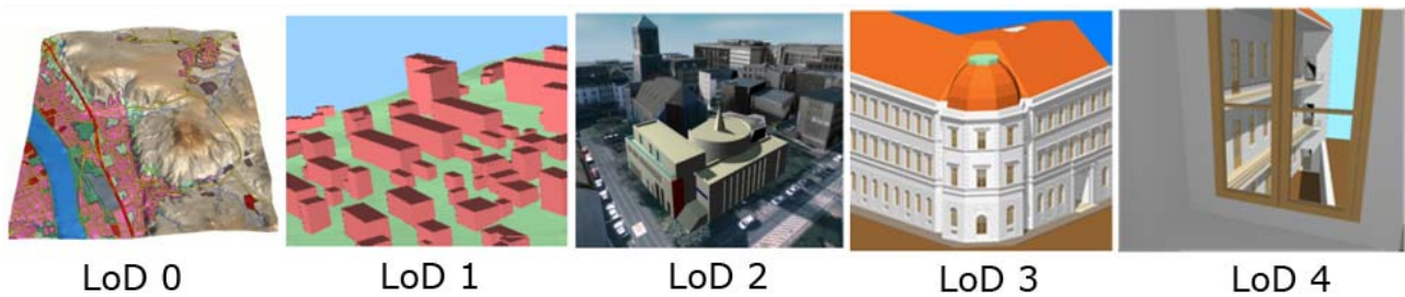
Fig. 2: The five Levels of Detail (LoD) defined by CityGML (Kolbe et. al., 2008).
