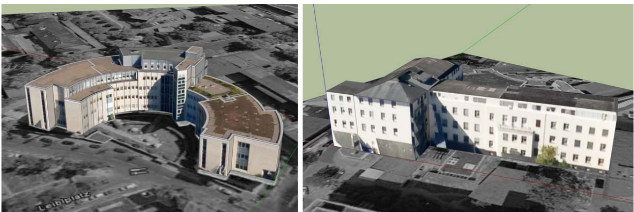
Fig. 4: Two example LoD2 buildings of the CampusGIS-3D model, created with Google building maker tool and visualized in Google Sketchup.
