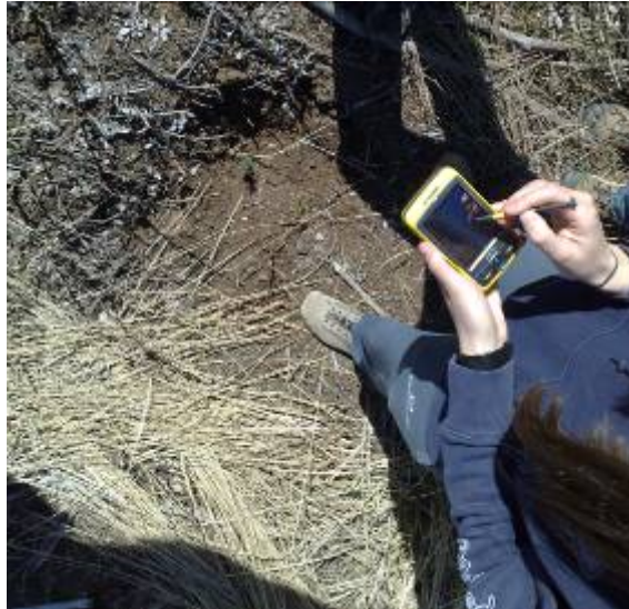
Figure 3. Measurement of spot for tree planting with Juno SC
