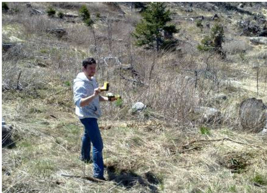
Figure 5. Surveyor, using Trimble Nomad field computer (below in his left hand) and Pro XT GPS receiver (above in his left hand), together with GeoBeacon radio modem (in the right hand)
