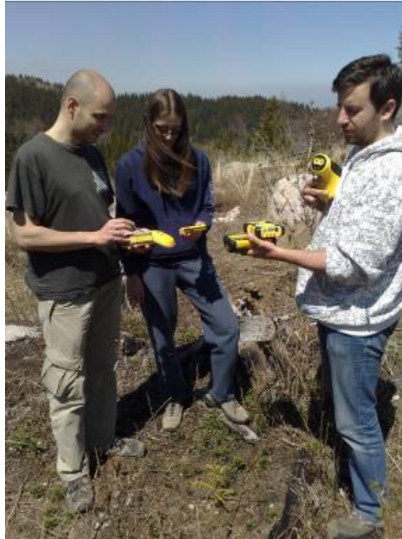
Figure 7. Mapping a planted tree by VRS (on the left), Uncorrected (in the middle) and MSK positioning methods
