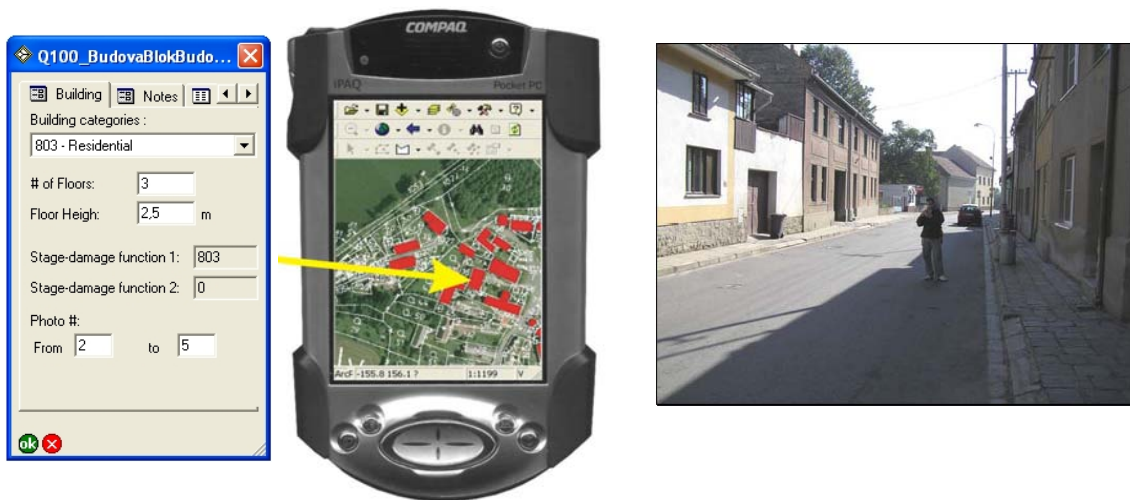
Fig. 10 Example of data collection on the structures in the floodplain to estimate the potential flood damage.
